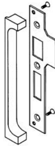
5. The striking plate rim secured to the striking plate. Left hand shown.
