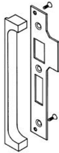
4. The striking plate rim can be fitted either side of the striking plate (and secured by screws shown) depending upon hand.
