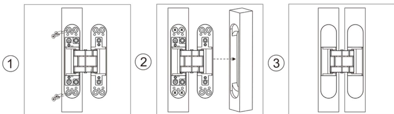
Put the hinge of frame end into the slotted door frame, to tighten with 4 pieces of 5mm wooden tapping screws.
