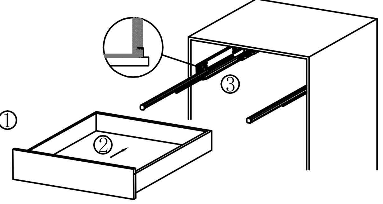
Front Connection With Height Adjustment Function
