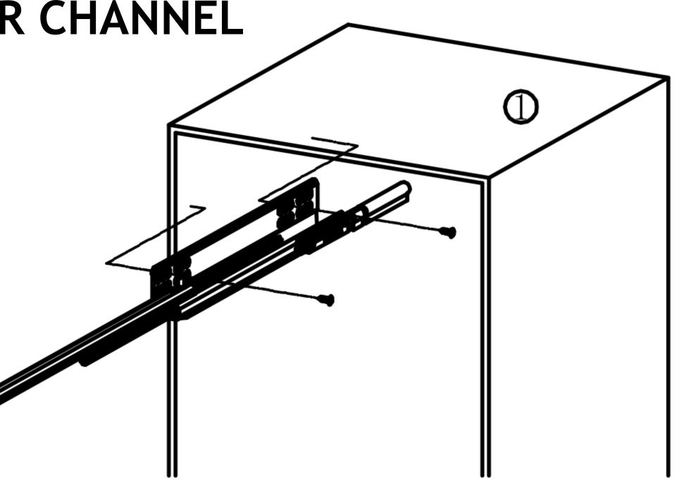
Step 1: Slide Mounting Place the drawer horizontally on the slide rail and gently slide it into position.
