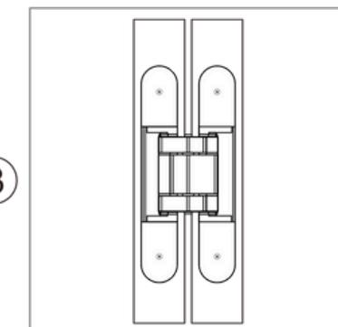
Fix the hinge of frame end and the door end, adjust the appropriate dimension, and finally tighten decorated cover plate.
