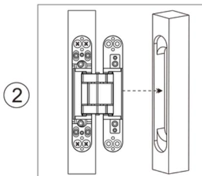
Put the hinge of door end into the slotted wooden door, Loosen the upper locking screws slightly if necessary, To adjust the height, to tighten with 4 pieces 5mm wooden tapping screws;
