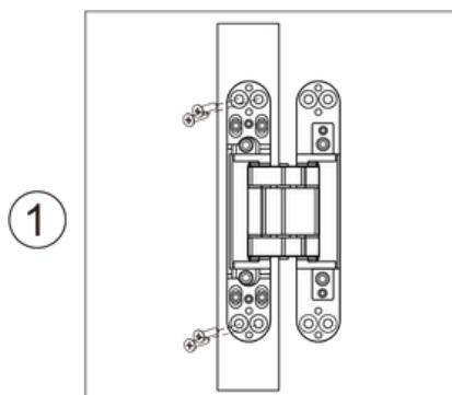
Put the hinge of frame end into the slotted door frame, to tighten with 4 pieces of 5mm wooden tapping screws.
